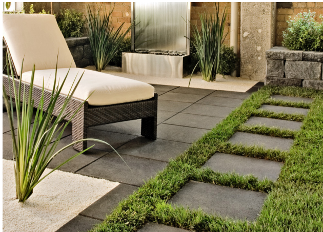
Surface type D - Patio pavers. Firth Chancery® 500Lx500Wx50D mm pavers or similar approved. Colour light grey 'Volcanic Ash' Permeable options available
