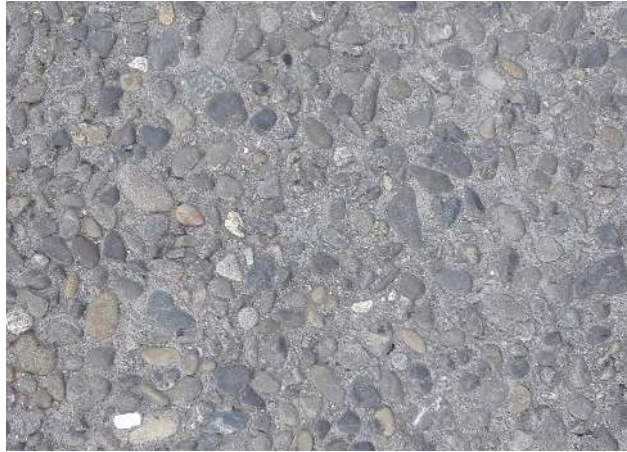
Surface type B - Exposed aggregate concrete - 16mm awatoto with awarua pebble 5% black oxide - decorative saw cuts tbc in detailed design.
